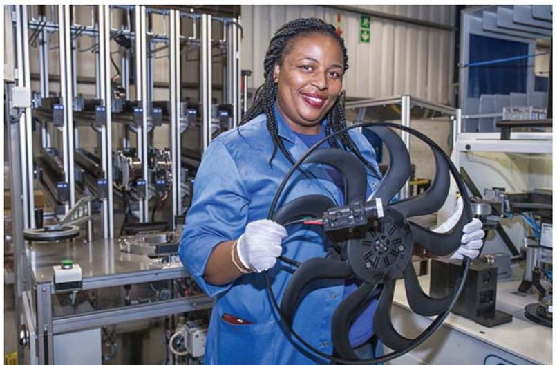
*Bongekile Myende, a MBZA employee holding up a fan motor assembly just after it has passed the balancing check*
